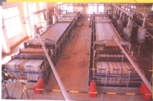
水平胶带式过滤机 series of horizontal belt vacuum filter 1.1~60m 2
