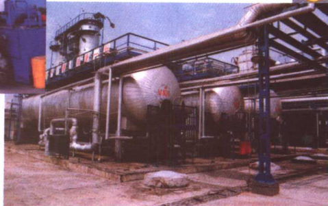
电脱盐成套设备 complete-sets of equipment for electric desalting 5,000kt
