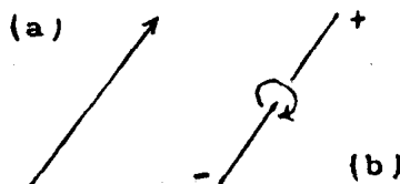
Fig. 1.3 Symbolic representation of vectors. (a) a polar vector, (b) an axial vector
