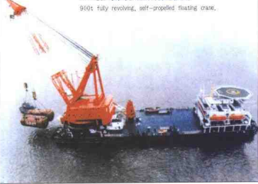
900吨全回转海上装卸打捞起重船。 900t fully revolving, self-propelled floating crane.
