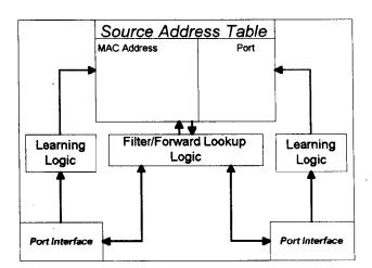
There are several key components in the forwarding logic of a LAN switch, as defined in the following list.
