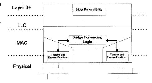
of the basic forwarding logic of the switch is needed. Figure 1.2 illustrates the logical model of the LAN switch (or bridge).
