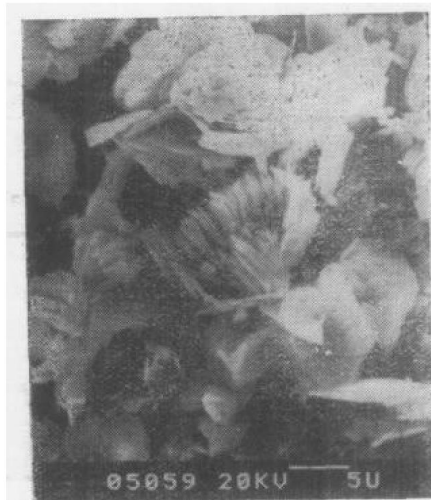
照片 4 成岩期孔隙中沉淀的高岭石，自形好，集合体呈书册状 扫描电镜×2500 photo 4 kaolinite deposited in the pores in diagenesis, euhedral, booklike aggregates SEM ×2500
