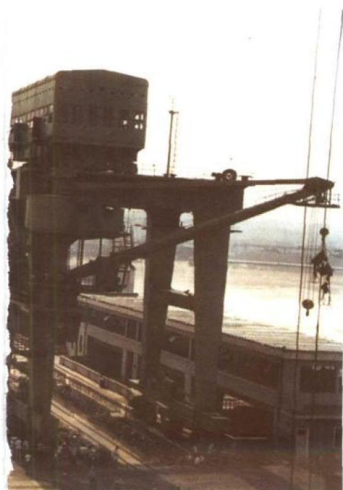
电站的2 × 250吨桥式起重机 Installed by Taiyuan Heavy Machinery Works in 1970s.
