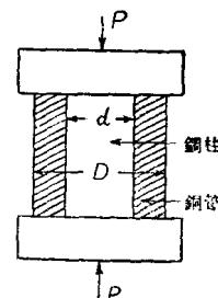
鋼的  $E_s = 2.1 \times 10^6 \text{ kg/cm}^2$ , 銅的  $E_c = 1.13 \times 10^6 \text{ kg/cm}^2$ .
