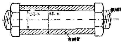
$$\begin{cases} \text{彈性係數} & \left\{ \begin{array}{l} \text{青銅 } E_b = 0.68 \times 10^6 \text{ kg/cm}^2 \\ \text{ 鋼 } E_s = 2.15 \times 10^6 \text{ kg/cm}^2 \end{array} \right. \\ \text{每 } {}^{\circ}\text{F 的熱膨脹係數} & \left\{ \begin{array}{l} \text{青銅 } \epsilon_b = 10.1 \times 10^{-6} \\ \text{ 鋼 } \epsilon_s = 6.1 \times 10^{-6} \end{array} \right. \end{cases}$$
