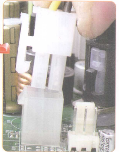
将CPU电源插头插入CPU电源插座
