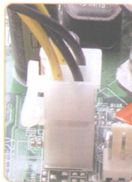
将CPU电源插头插入CPU电源插座
