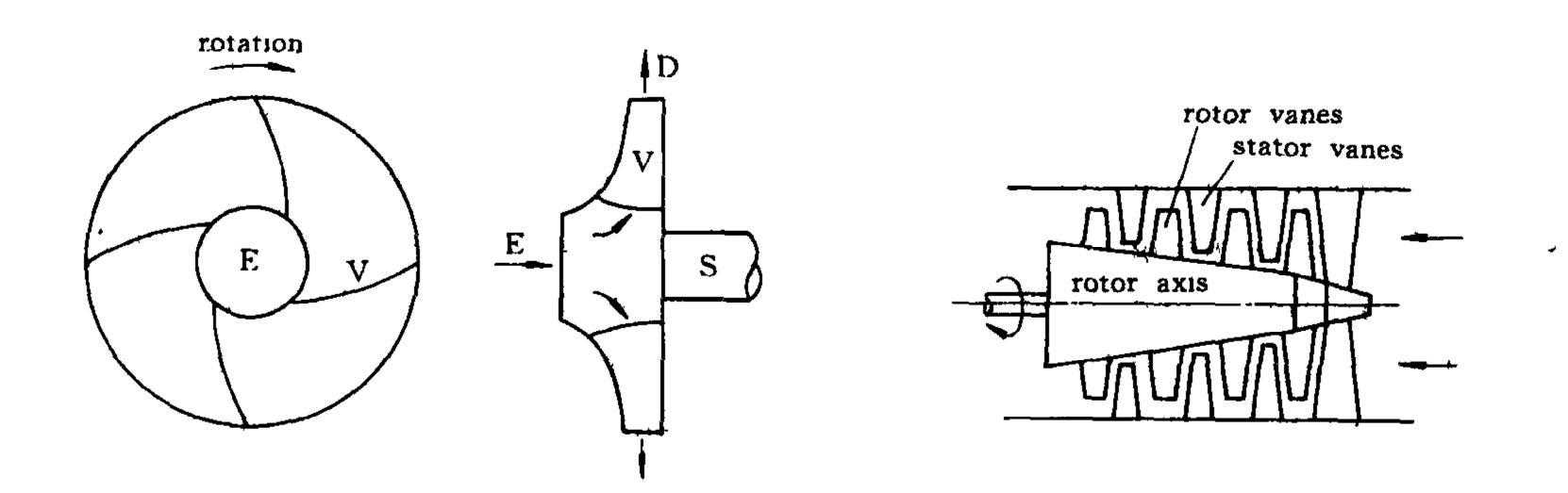
Fig 3. 1 Pump impeller
