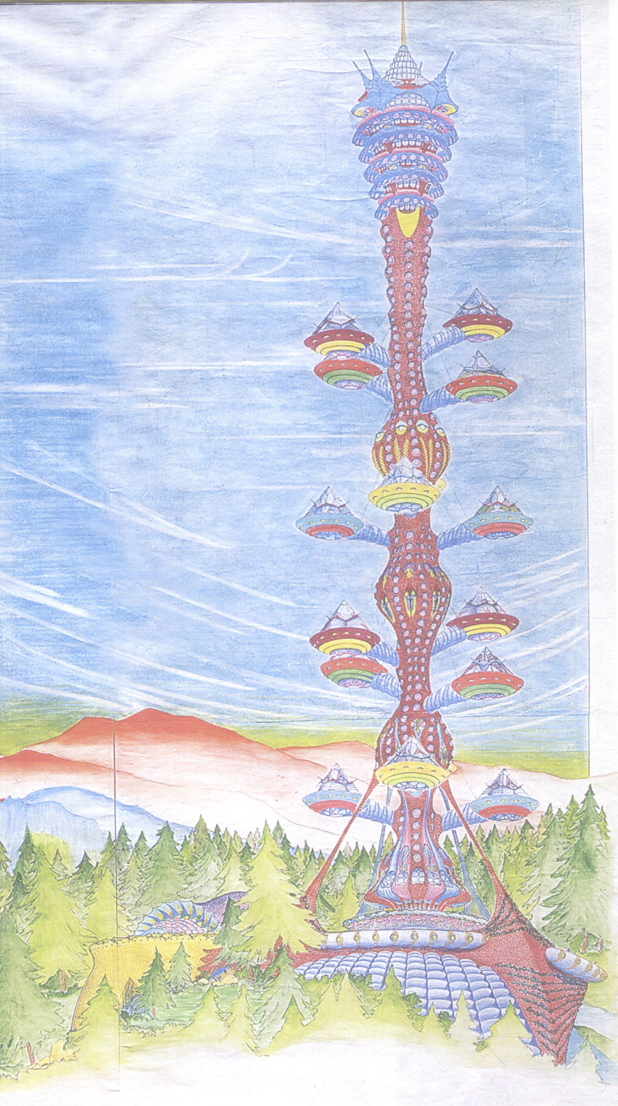
图4 美国国家公园服务部的宿舍、研究室和观光塔。每组宿舍群包括有四间三个床位的宿舍，分别悬挂在中央的不锈钢核上。 Apartment residence, research laboratory and recreation tower, for the National Park Service, USA. Each apartment "pod" contains four, three-bedroom apartments suspended from a central Cor-Ten rustproof steel core.
