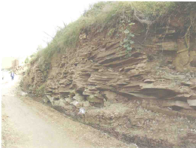
滑坡下伏滑床砂岩呈层状碎裂岩体， 富水性好 Laminar sandstone at the base of the sliding mass initially large amount of water
