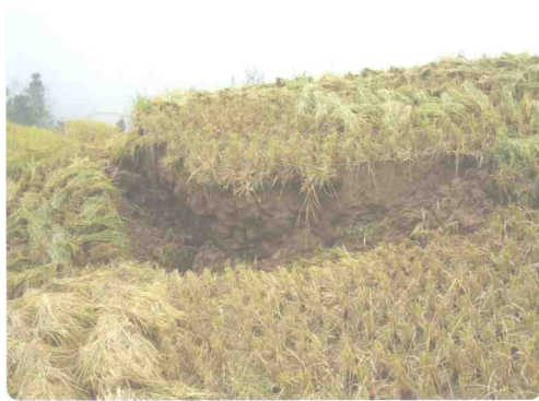
稻田被毁, 田水入渗促使滑动加剧 Rice field destroyed by sliding, resulting in water seepage and exacerbating landslide
