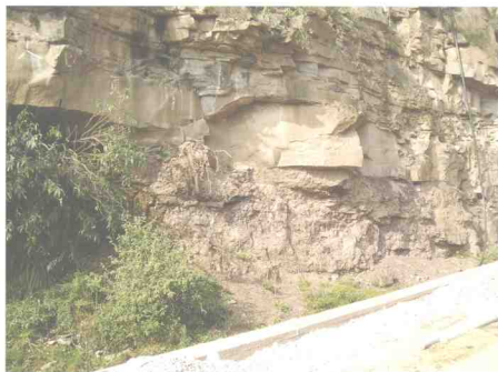
滑坡下伏滑床为砂岩泥岩互层结构 Interbedded sandstone and mudstone at the base of the sliding mass
