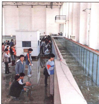
水港系學生港口測波實驗課 The students in the Department of Harbor and Waterway making wave-testing experiment
