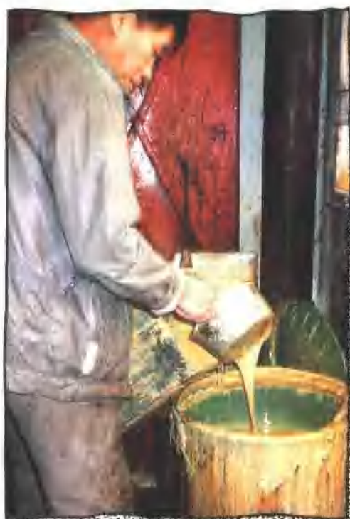
Solvent vaporises when mixing and using adhesives.
