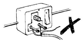
Electrical appliance should be protected against electric shock by proper earthing and earth leakage circuit breaker. Electric cable and appliance should be checked regularly. Damaged cable and mal-functioning appliance should be taken out of service immediately.
