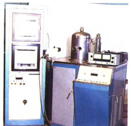
Auto-recording equipment for measuring thermal emissivity
