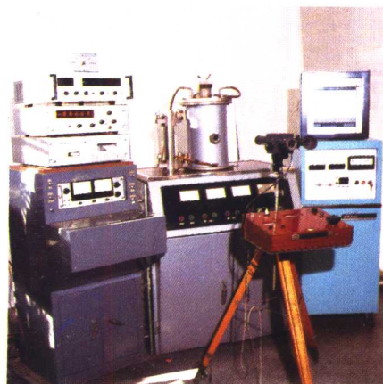
Auto-adiabatic equipment for measuring specific heat
