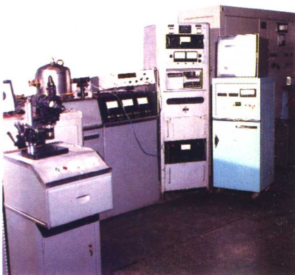
Laser pulse equipment for measuring thermal conductivity
