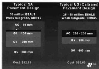
Figure 7 A Comparison of Typical Nominal Pavement Structures in South Africa and California (after Nordengen 2002)
