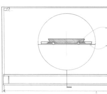
Rollers enable the parallel rule to move freely across a drawing surface.
