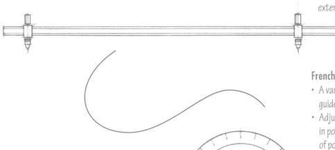
• Even larger circles can be drawn by appending an extension arm or using a beam compass.
