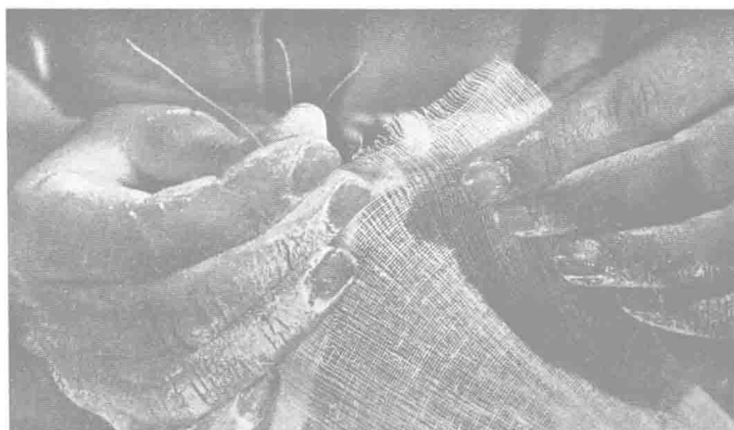
FIG. 1.—Three threads are drawn off each edge of the muslin strip.
