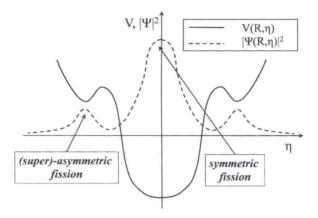
Fig. 2 Potential of a symmetrically fissioning nucleus as a function of the mass-asymmetry  $\eta$  (solid line). The collective wave function squared  $|\Psi(R, \eta)|^2$  as a function of  $\eta$  at fixed R (dashed line)
