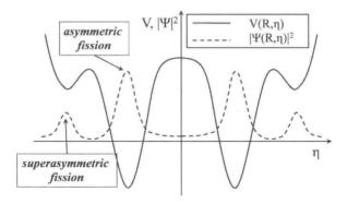
Fig. 3 Potential of an asymmetrically fissioning nucleus as a function of the mass-asymmetry  $\eta$  with additional possibility of superasymmetric fission
