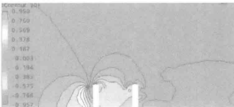
(a) Wind pressure coefficient of center vertical vertical profile
