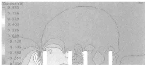
(b) Wind pressure coefficient of center vertical profile when S = 0.15D
