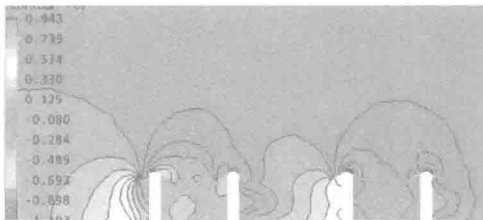
(c) Wind pressure coefficient of center vertical profile when S = 0.75D
