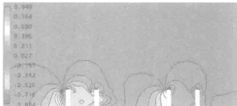
(d) Wind pressure coefficient of center vertical profile when S = 0.75D
