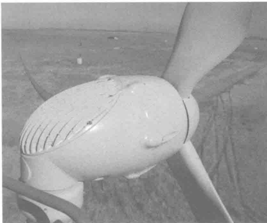
Figure I.3 The development of permanent magnet alternators has provided improved performance and reduced maintenance.
