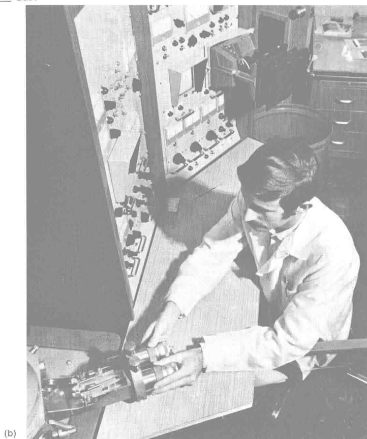
Figure 1-1. Modern microscopes. (a) Modern compound light microscope. Since microscopes of this kind use light, they cannot resolve structures smaller than 0.3 micrometer. This limitation is the result of the relatively long length of visible light waves. (b) Modern electron microscope. Instead of light, this instrument uses a beam of electrons. Since the wavelengths of electrons are about 1/100,000 that of the normal wavelength of white light, an electron microscope can magnify objects up to 200,000 times (a: Courtesy of Tasco Sales, Inc., Miami, Fla., b: Courtesy of RCA Laboratories, Princeton, N.J.).
