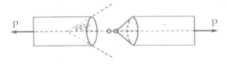
Shear strength < Tensile strength ≤ Compressive strength
