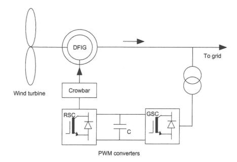
Figure 1.1 Type-3 wind energy system.
