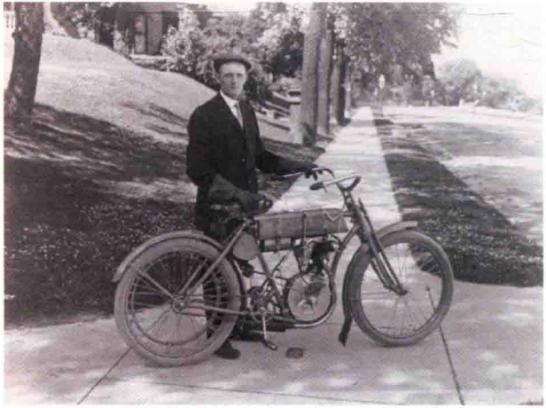
Figure 1-12 The first V-Twin built by Harley-Davidson had 7 horsepower and was built in 1909.
