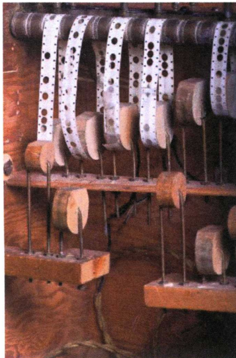
A Lehmer sieve, which is a primitive digital computer once used for finding primes and solving simple Diophantine equations.
