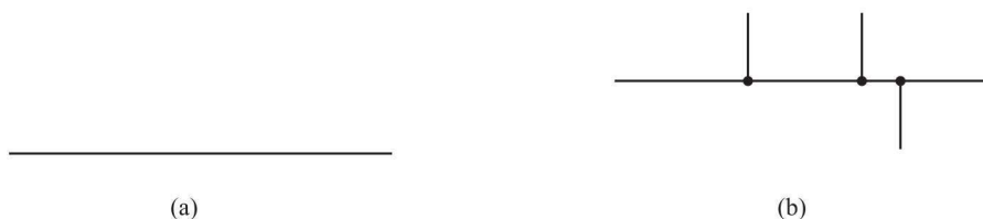
Fig. 1-4 Wire (a) Wire; (b) Wires joined
