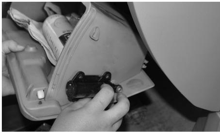
A black and white photograph showing the glove box being pulled out of the dashboard. A hand is using a screwdriver to remove a screw from the back of the glove box. |
