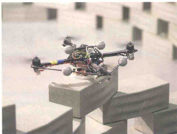
Fig. 1 The complex structure of the 1:100 installation has been assembled by autonomously flying “quadcopters” which land on a platform to pick up building elements and then set them down precisely on top of one another (Image by François Lauginie)
