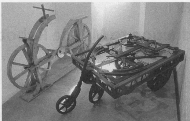
Fig. 1.1 Model of a bicycle and a programmable cart built based on Leonardo da Vinci's notes.
