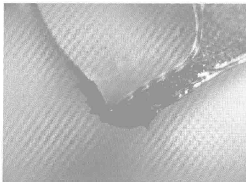
Fig. 2 Migratory plasticizers from PVC-P made bitumen softer
