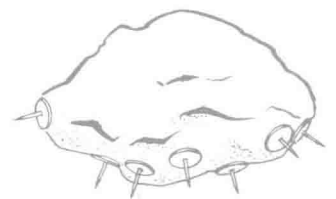
Figure 1-3 The attraction of iron tacks by a lodestone.
