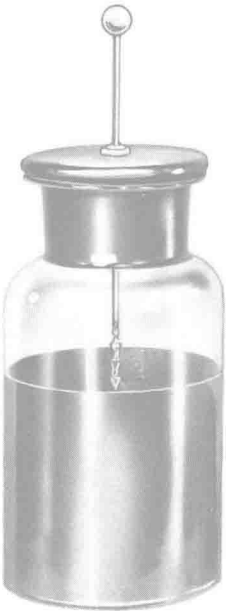
Figure 1-10 A Leyden jar. (Courtesy Sargent-Welsh Scientific Co., Skokie, Ill.)
