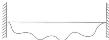
Figure 1.10 A flexible beam with infinite degrees of freedom.
