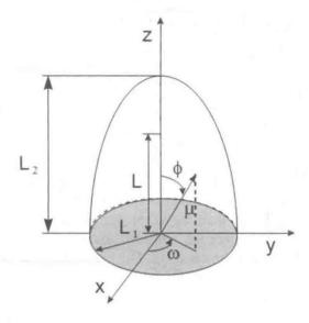
Fig. 2 Prolate spheroidal coordinate system
