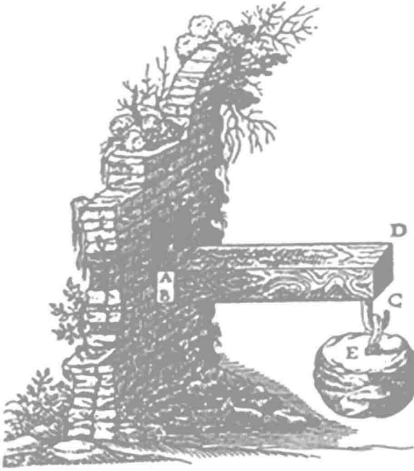
Fig. 3 Galileo's depiction of a beam (1638, p. 114)
