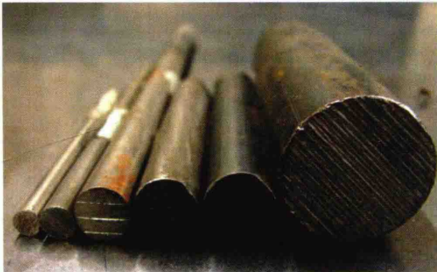
c. Round bar, also referred to as rod, is identified by its diameter. Example: 1/4" rod.
