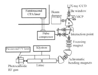
Figure 4. System configuration of laser-Compton X-ray source
