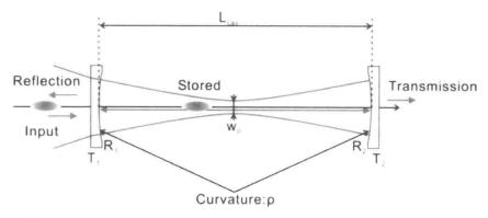
Figure 2. Schematic of laser storage enhancement cavity of Sakaue
