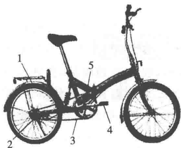
1-后轮; 2-飞轮; 3-链条; 4-踏板; 5-链轮
