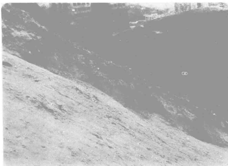
Plate 10 Landslide III showing shallow depth of slide and layering parallel to slope
