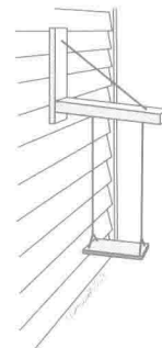
Figure 1.4f Swing fixed to a wall
