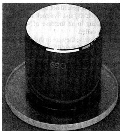
Fig. 1-4 The international 1 kg standard of mass, a platinum–iridium cylinder 3.9 cm in height and in diameter.
