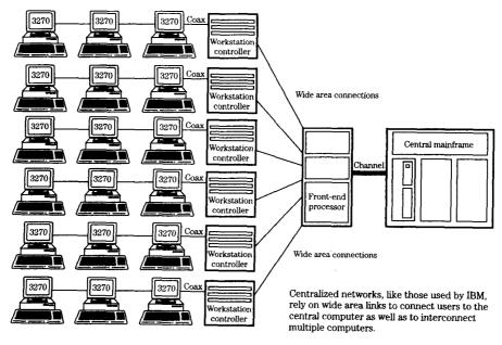
Shown here is a typical IBM terminal network.
