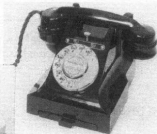
The 300 model desk telephone (1937) – bell included in the telephone for the first time
