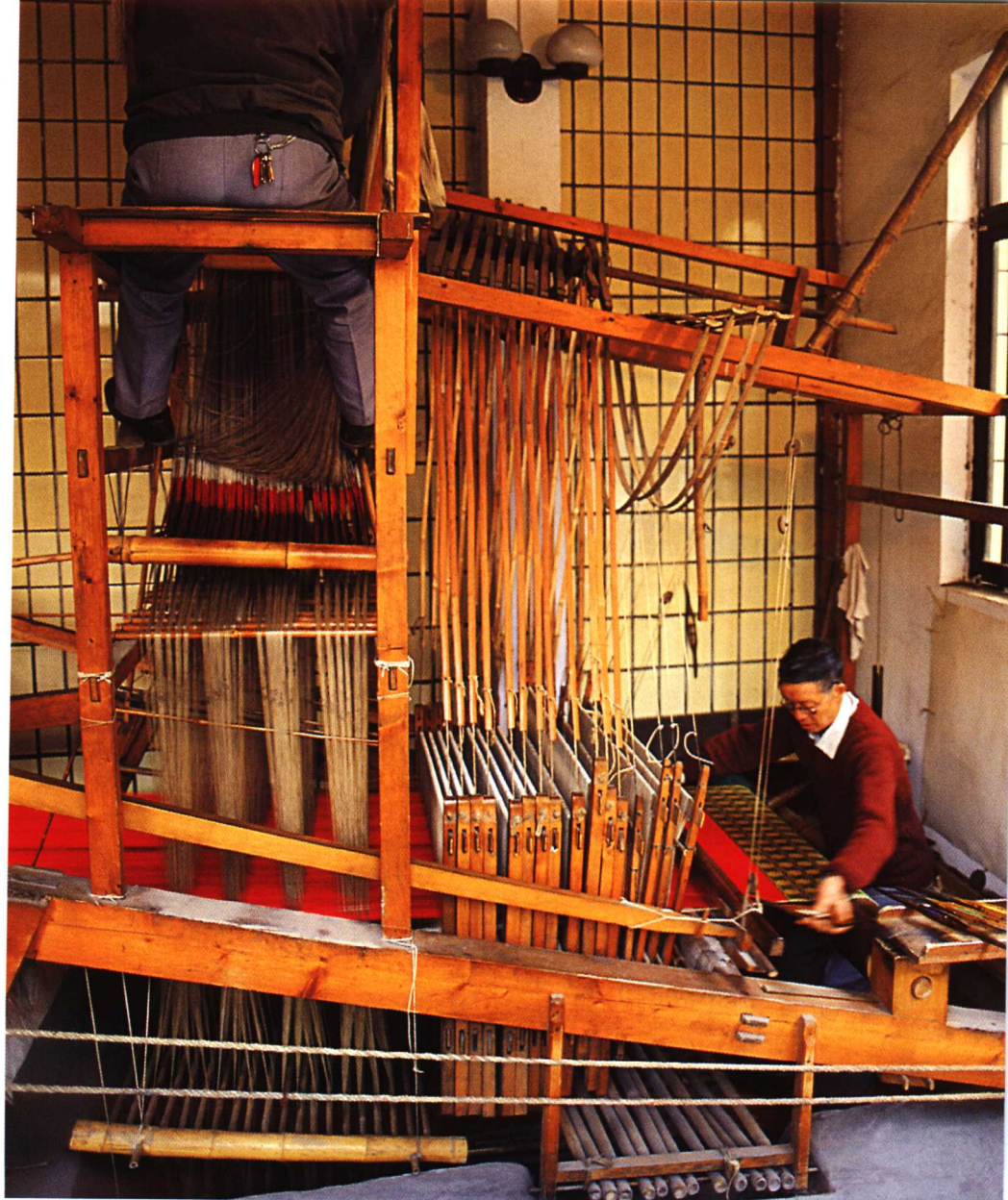
Demonstrating the Qing Dynasty hualou loom.
