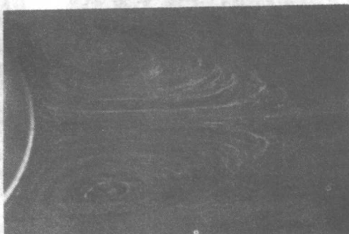
Figure 4.12.8. Streamlines, in an axial plane, of steady flow (from left to right) past a sphere of radius a (from Taneda 1956 b ); R = 2aU/\nu .
