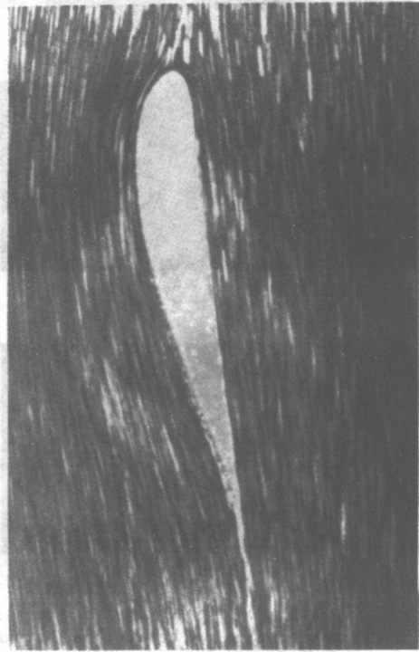
Figure 5.11.1. Flow from right to left past an aerofoil (a) aligned roughly with the stream, and (b) not so aligned. (From Prandtl 1930.)
