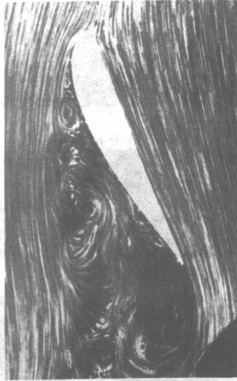
Figure 5.11.1. Flow from right to left past an aerofoil (a) aligned roughly with the stream, and (b) not so aligned. (From Prandtl 1930.)
