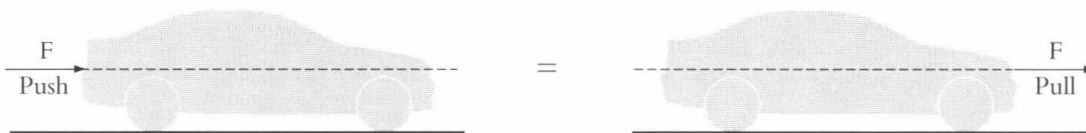
Figure 1.11 Principle of transmissibility
