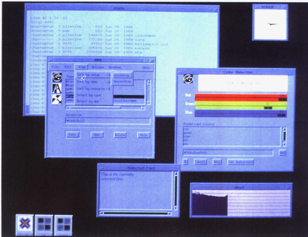
Plate 9. The OSF/Motif user interface. The color slider bars are used to define colors for use in windows. Notice the use of shading on the edges of buttons, menus, and so forth, to create a 3D effect. (Courtesy of Open Software Foundation.)
