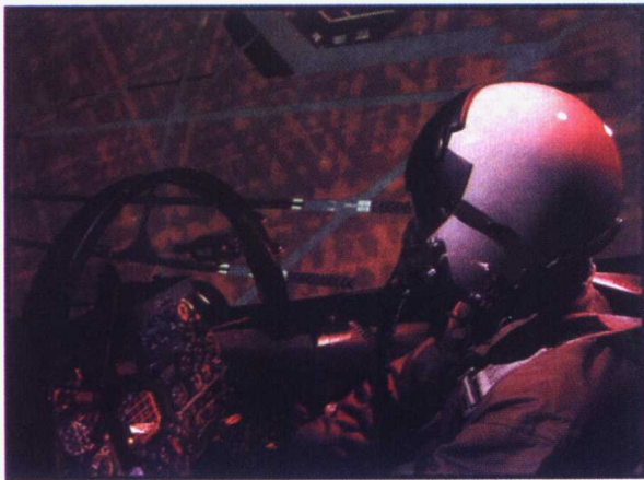
Plate 4. (a) The cockpit of an F5 flight simulator; the pilot's view is projected onto a dome surrounding the cockpit. (b) The view from the cockpit of the flight simulator. The fighter jet is modeled geometrically, whereas the terrain is photo-textured. (Courtesy of R. Economy, General Electric Company.)
