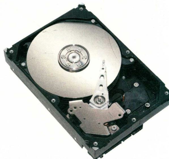
FIGURE 1-4 Hard disks are self-contained devices. The hard disk shown here must be installed in the system unit before it can be used.
