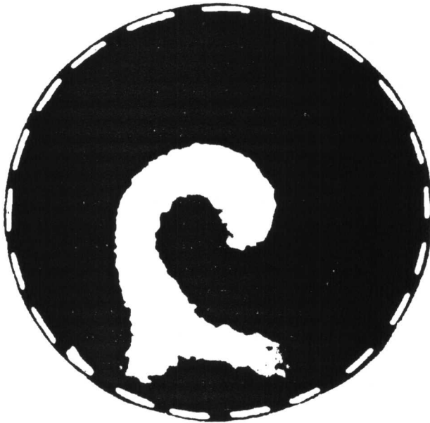
Fig.5. A photograph of a radial segment of the arc showing small-scale arc-wall shunting.
