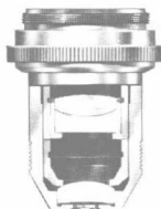
Cross section of low power objective, 10X.
